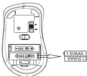
3. Turn the power switch to "on", press and hold the 'connect button' on the bottom of the mouse for three seconds, you will now see the scroll wheel flashing blue. The mouse is now in pairing mode.
