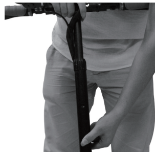
Step 7 Adjust the Position Button with one hand, and hold on the T-bar with the other
