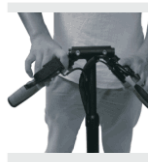
4/Press down the left and right handlebars
