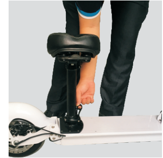
Step 4 Push outward the folding handl
