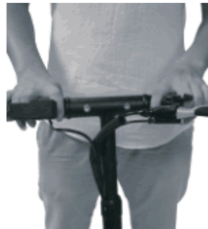
3 Pull outward the left and right handlebars
