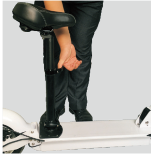
Step 1 Force apart the Fast Fold Pipe Clamp
