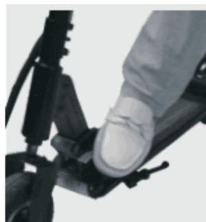
6 To lock the folding mechanism, place the scooter on the ground, push joint release lever down.
