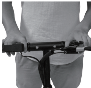
Step 6 Push inward the Sliding Sleeve
