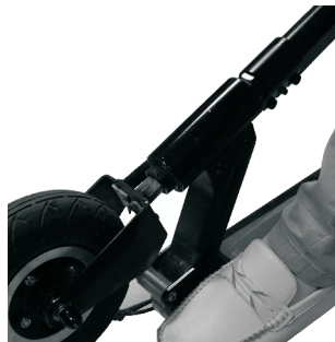
Step 2 Unfold the Ride Bar, stabilize the Footplate with the left leg, and uplift the Front Tube with both hands
