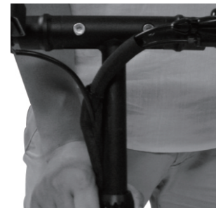
Step 8 Rotate tightly the nut clockwise
