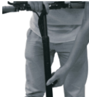
2 Press spring-loaded buttons, Insert T-bar into the fork until its bottoms.
