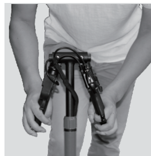
Step 3 Slightly push forward until a crash sound is heard
