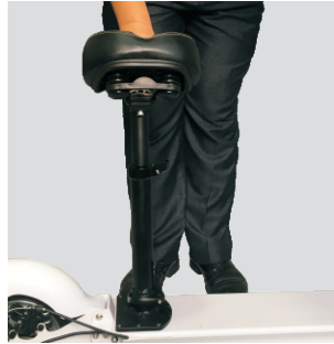
Step 2 Rotate the seat 90 degrees
