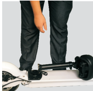
Step 6 Lay the seat tube down to the ground, straighten the scooter, slightly step downward on the folding handle with the left leg
